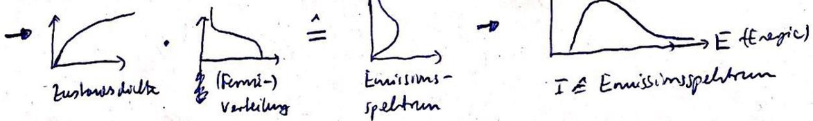
$$I(E) \sim \sqrt{E - E_g} e^{-\frac{E}{k_B T}} \quad \& \quad E = E_g + \frac{1}{2} k_B T$$
